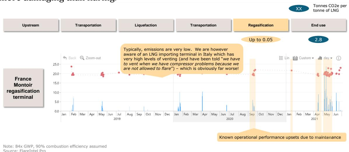
**Figure 5: Flaring associated with France's Montoir regasification terminal. Whilst flaring is generally quite low, it is likely avoidable (as it is in many other regasification terminals). Flaring is, however, much more preferable than venting, which has been directly observed at an Italian regasification terminal.**
