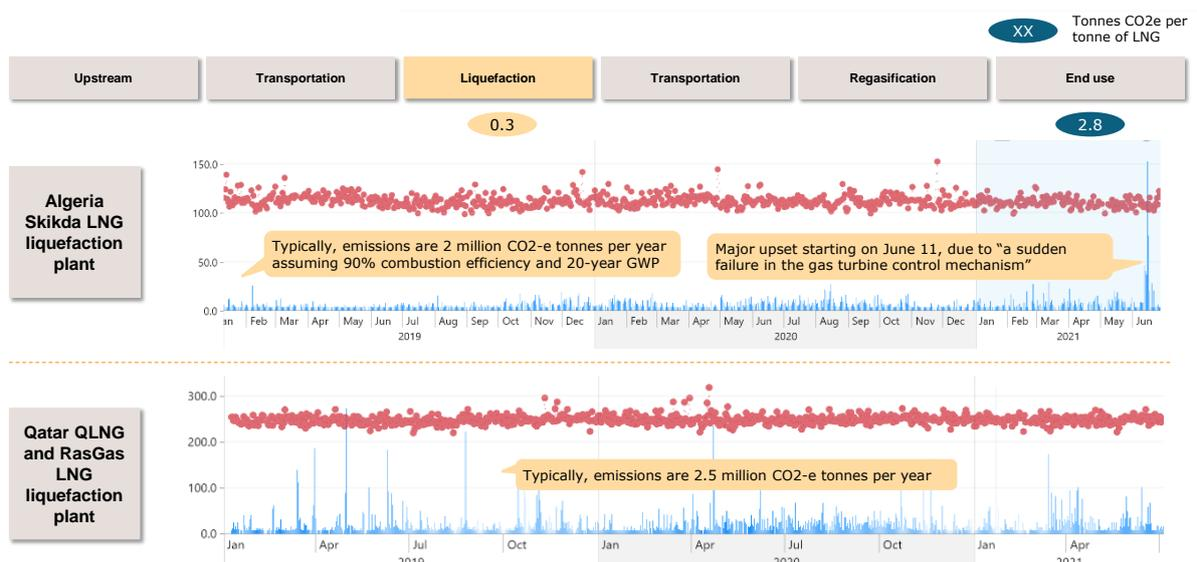
**Figure 4: Flaring associated with Algeria's Skikda liquefaction plant, and Qatar's liquefaction plants. Both facilities generated around 2 million CO<sub>2</sub>-e tonnes per year, assuming 90% combustion efficiency of the flare, and a 20-year GWP. Both facilities have major periods of "upset" conditions, which are likely driven by issues around equipment maintenance.**
